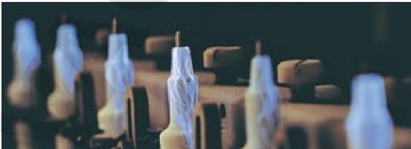
Testing an insulator at 40,000 Volts.
